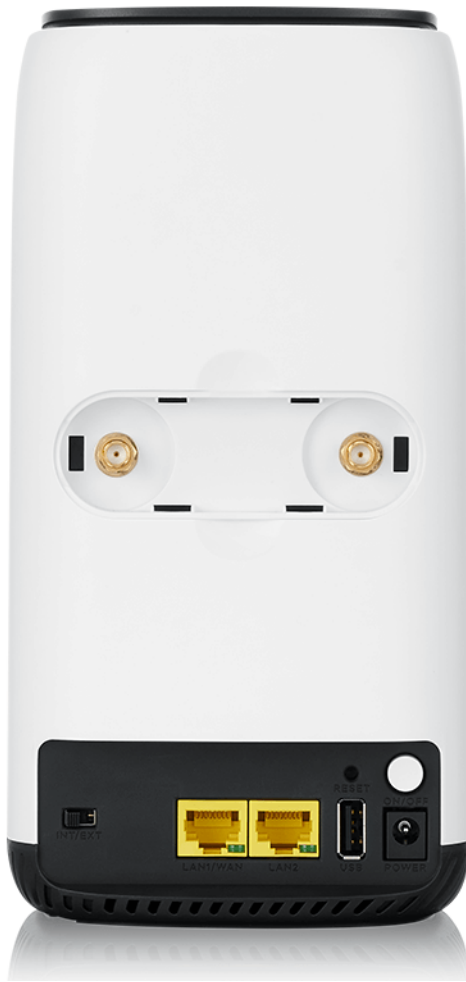
Figure 18 Antenna Ports on the Rear Panel (NR5101)
